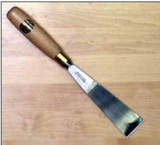
I have to use the flattest sweep possible to carve the background very smooth while leaving it subtly 'tooled'; a gouge just flat enough not to be a straight chisel.
