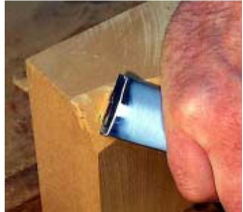
I am so convinced of the usefulness of this inner bevel on flat gouges that, rather than let the carver have to put one on, as is the case with all other makes of carving tools, that I asked Ashley Iles to include it in these new flat gouges.
