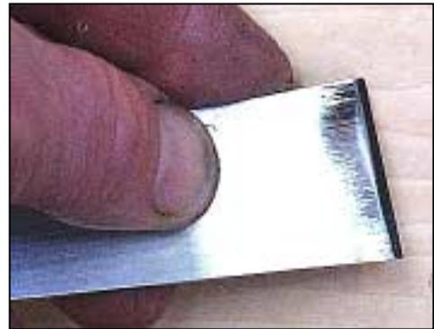
It is these 3 features: the *thinness* of blade, *flatness* of sweep, and *inner bevel* that make these tools unique, and so useful for finishing surfaces.
