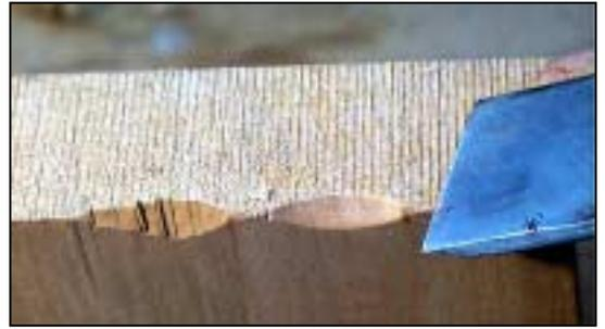
The result will depend on the shortness of the bevel, the thickness of the blade and whether the heel (the angle between bevel and blade) is rounded or not.
